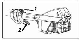
Release the On/Off switch to switch it off.
