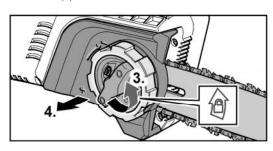
Place saw chain around the saw rail starting on the upper part of the rail. Slide the chain in the slot around the saw rail. When attaching the chain, ensure that it is in the correct running direction.
