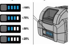
The indicator goes out after 3 seconds. If one of the LEDs flashes, the battery must be recharged. If none of the LEDs light up after the button is pressed, the battery is faulty and must be replaced.
