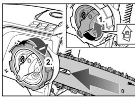
Detach the handwheel (3) and remove the chain cover (4).
